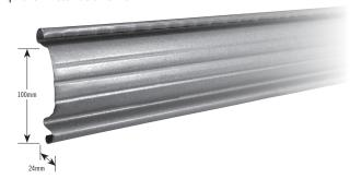
High tensile G550 continuous roll formed, interlocking, coated Galvabond® steel slats. Nominal effective pitch of 100mm with 3 small ribs. Zincalume® coating of not less than 150g/m². Moulded nylon clips fitted to end of alternate slats by means of three nylon rivets.
