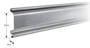
1.2mm, continuous roll formed, interlocking, coated galvanised steel slats. Nominal effective pitch of 100mm. Zinc coating of not less than 275g/m $^2$ .
