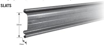
0.6mm, continuous roll formed, interlocking, coated galvanised steel slats. Nominal effective pitch of 100mm. Zinc coating of not less than 275g/m².
