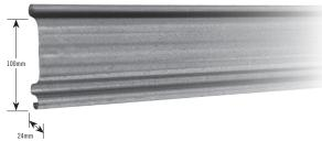
0.8mm, continuous roll formed, interlocking, coated galvanised steel slats. Nominal effective pitch of 100mm. Zinc coating of not less than 275g/m².
